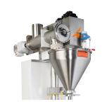
HORIZONTAL SCREW CONVEYOR: Optional Model/HSC, which is mounted directly to the side of your your semiautomatic auger filler head, supplying a steady flow of product, reducing labor and improving machine efficiency.
